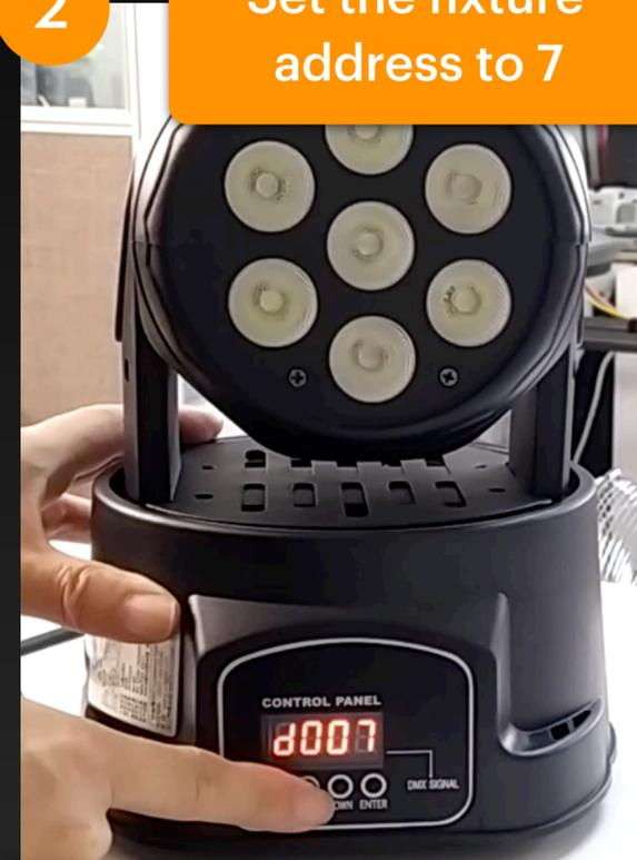
After modifying the address of the lighting fixture, the channel number it occupies on the DMX bus will also change accordingly. Take this moving head light as an example, when the address is changed to 7:
